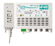
**Three-input OPT-MBJ optical transmitter** for distribution of band 3, UHF and full IF-IF signals on a single fibre. Laser optical output level of 5dBm, wavelength 1550nm. (dimensions 135x82x39mm)
